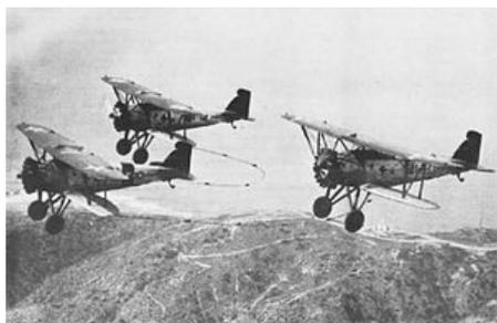
Fighting Six B traded their F6Cs in for the new air cooled Boeing F2B-1 fighter planes. The F2B-1 was the next step in the evolution of the development of dive bombing which the squadron was working to perfect. This aircraft was mounted with two forward firing thirty caliber machine guns and could carry five twenty five pound bombs. It could fly faster and higher than the F6C. Curly
